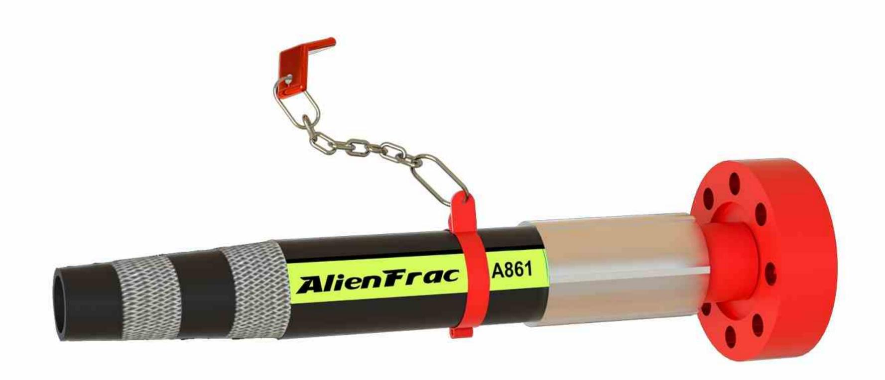
**Tube:** synthetic rubber **Reinforcement:** multi-layer of high tensile synthetic textile **Cover:** high performance Abrasion Resistant Cover **Connectors:** swaged fittings, integral union or flange **Application:** Designed for discharge use of petroleum based fluids, dilute acids, chemical and abrasive slurries used in oil and gas well stimulation and fracking.
